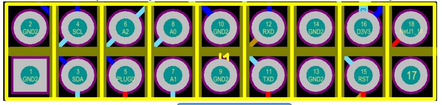
Fig 8. Each Pin Definition of IO
