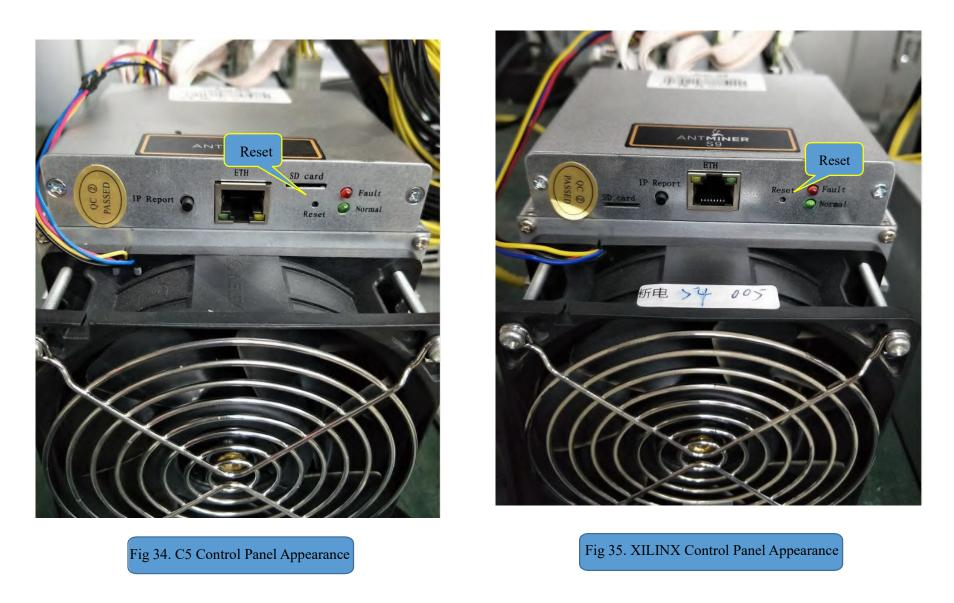
Factory reset of C5 control panel: long press "RESET" key for more than 5 seconds after miner works; when the red light is on, reset miner successfully. Factory reset of XILINX control panel: In off mode, long press "IP Report" for more than 5 seconds and then let go, to complete factory reset. If factory reset has no effect, enter control panel maintenance process.
