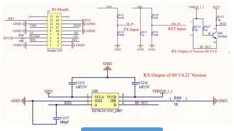
Fig 9. Each Division Voltage of IO Signal of S9
