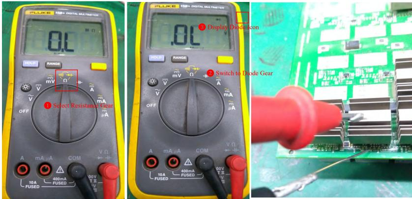
1. Firstly, switch the multimeter to resistance gear, and then press yellow button to shift gear, until the screen displays the diode icon, which means multimeter has tuned to diode gear.
