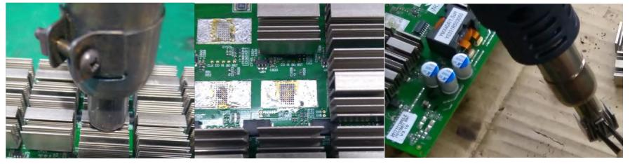
Disassemble the cooling fin on the back, heat the cooling fin on the back until the temperature is high enough to melt tin, and then use tweezers to remove it. In assembly, heat outside first until the temperature is high enough to melt tin, place the cooling fin on the pad and press.
