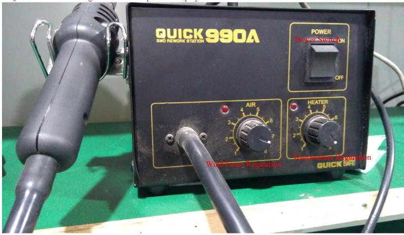
I. The Application Method of Heat Gun: firstly, switch on and adjust to proper temperature, heat gun with temperature display is recommended to buy, about 360°C in general, depending on the specific environmental temperature, and then adjust to proper wind force. Switch off the power when not in use for a long time. This product will produce high temperature, beware burn! When switching off, heat gun will not
