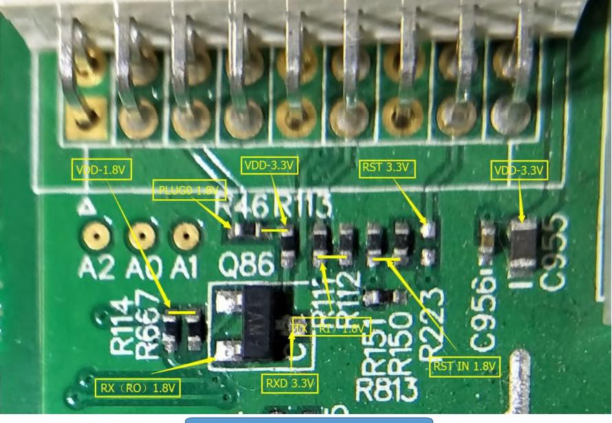
Fig 10. Each Division Voltage of IO Signal in 1.9 Version
