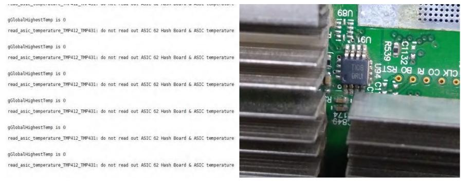
In this situation, firstly check the model of the temperature sensor IC beside chip 62 as above Fig, to ensure the consistency of the temperature configuration file in hashboard tester TF card and the temperature sensor IC model of tested board. If they are inconsistent, replace temperature configuration file and use tester to have a power-on test again.
