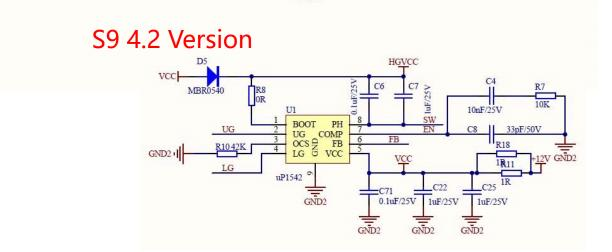
Fig 15. DC-DC Schematic Diagram
