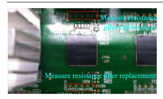
4. Replace a chip and let it cool, then measure the 10 test points on the two sides of the chip, to see whether their resistances are normal. Have power-on test when all resistances are normal. Otherwise, reweld the chip until resistances under measurement are normal.
