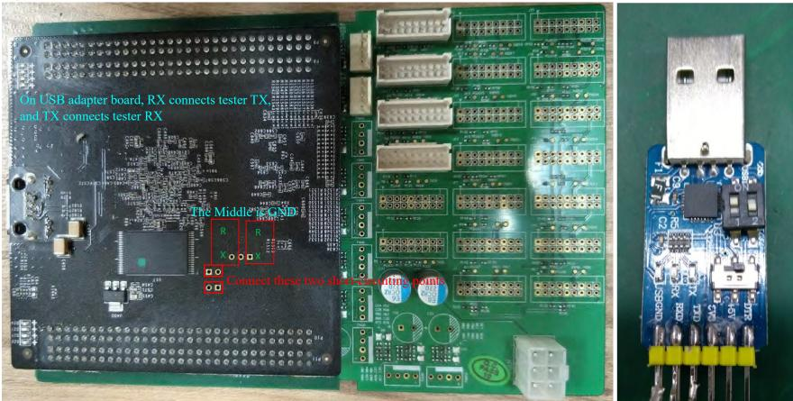
III. Install the drive to transfer USB to TTL in computer, and then transfer USB to TTL adapter board and insert to computer USB interface. PL2303 drive download CP 2102 drive download, open Hyper Terminal directory.
