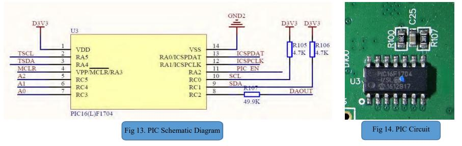
When PIC works, it needs to control and send a heartbeat signal every minute. Without heartbeat information, PIC will be closed after one minute. PIC pin 1 is VDD 3.3V, pin 14 is GND, pin 9 and 10 are I<sup>2</sup>C bus wire that connects IO mouth to control panel, pin 5, 6 and 7 are PIC addresses; pin 4 is PIC 3.3V; pin 8 is the FB output of PIC, and controls DC-DC voltage; pin 11 is EN signal that PIC outputs, and controls DC-DC operational status.
