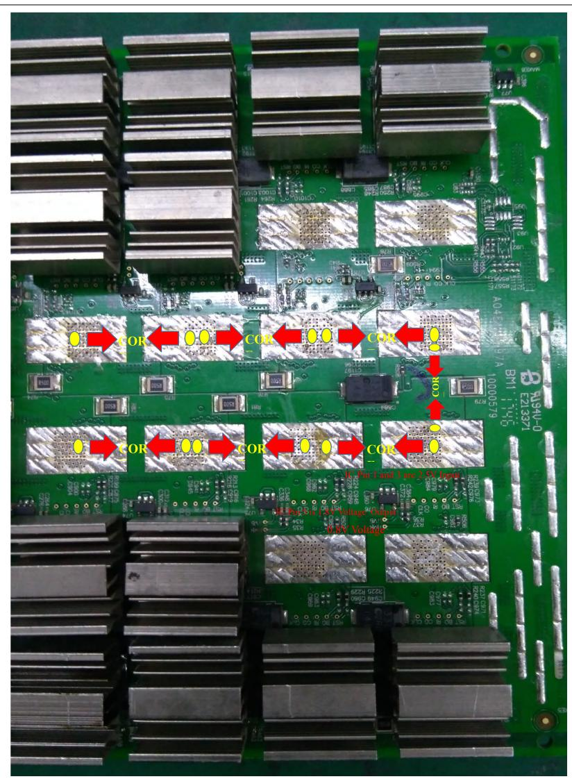
Fig 7. Test Points around Chip and Each Voltage
