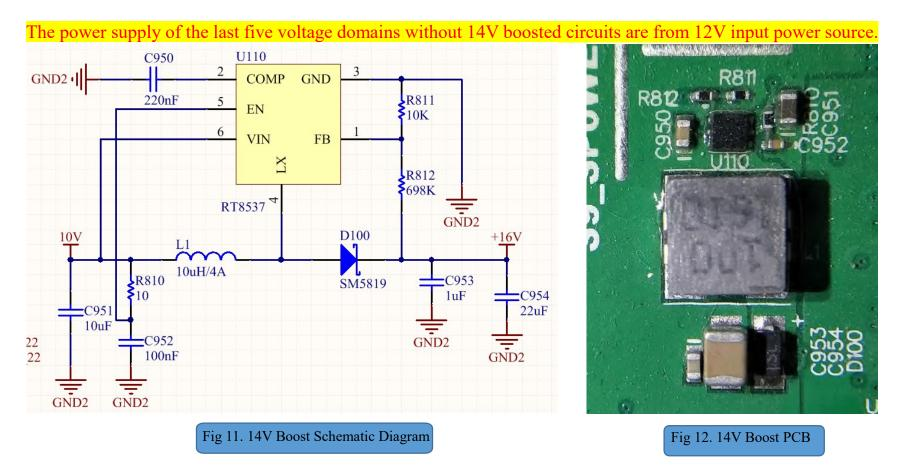
Note: the voltage anomaly of booster circuit often causes the LDO damage of the last 5 voltage domains of hashboard, and also causes chip damage easily. And the anomaly of boost voltage is often caused by the oxidation of U110, R812 and R811.
