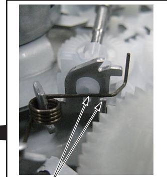
One end of the spring is engaged beneath the resin flange and plate bend. Fig. 2a Original engagement position
