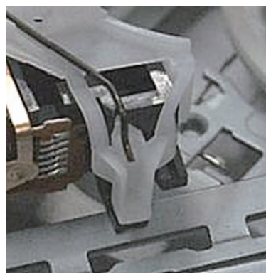
[Improper assembly] The chassis is not properly pinched by the PU case and PU rack.
